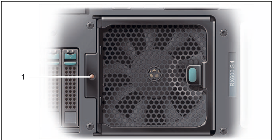
Figure 16: Fan status indicator (right fan module)
